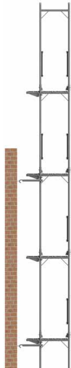
Figure 45: Free-standing scaffolding level as an intermediate state during the erection of buildings.
