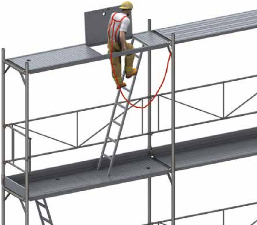
Figure 22: Safeguarding with the PSAgA prior to the entering of the highest scaffolding level.
