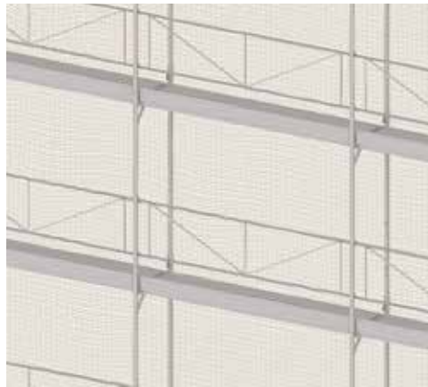
Figure 42: Cladding with tarpaulins.
