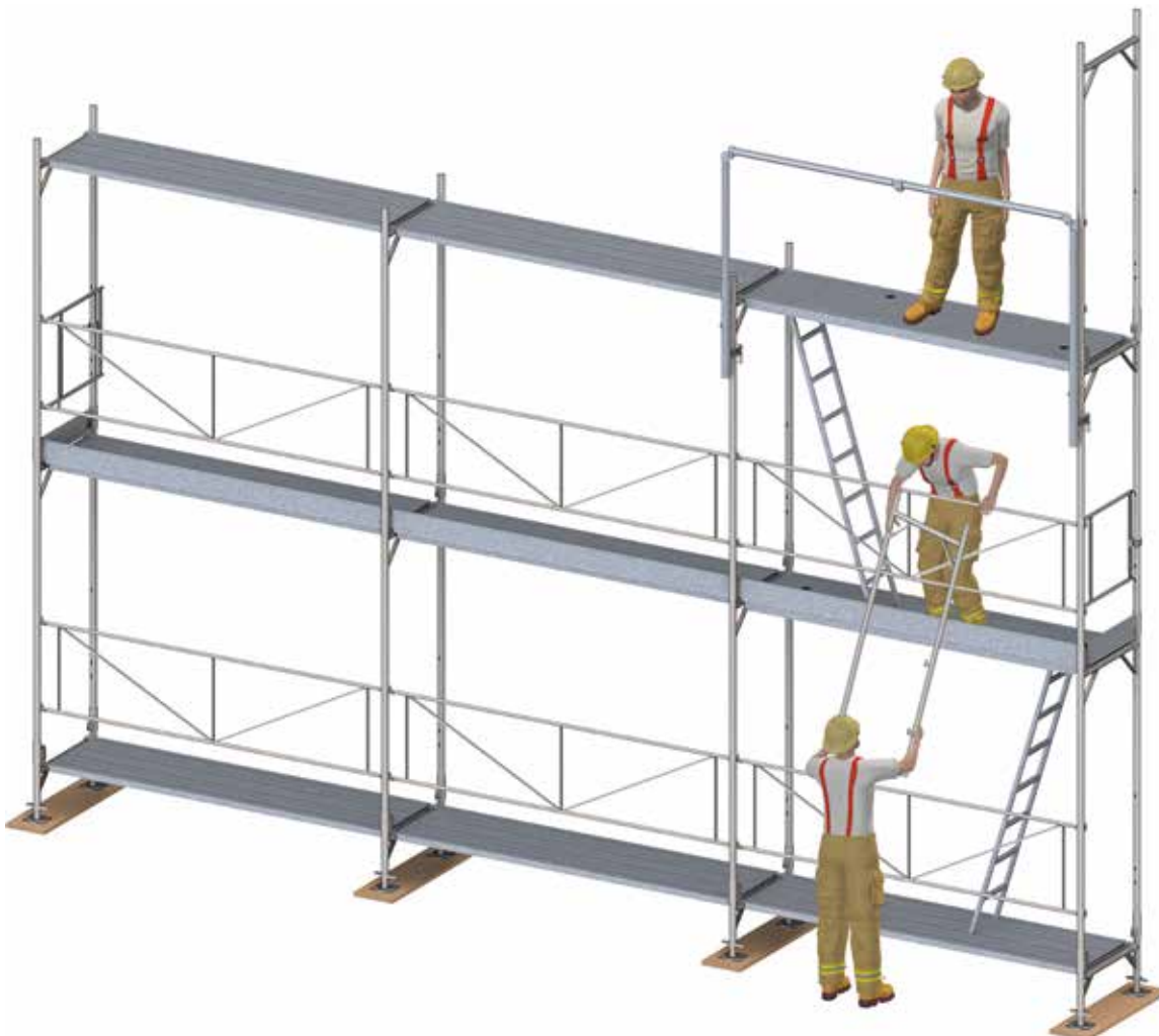
Figure 13: Example of manual usage of the components and assembly on the highest scaffolding level.
