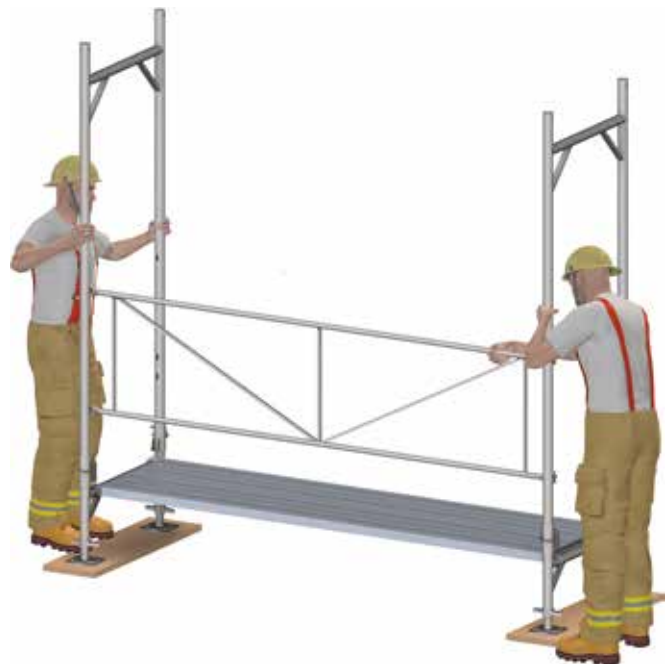
Figure 3: Assembly of the first scaffolding bay.
